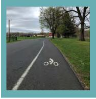
**Description:** A portion of the roadway that has been designated by striping, signage, and pavement markings for the preferential or exclusive public use by bicyclists. Bicycle lanes are located directly adjacent to motor vehicle travel lanes and operate in the same direction as motor vehicle traffic.
