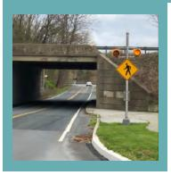
**Description:** A flashing warning device can be used in combination with pedestrian crossing signs and a marked crosswalk at uncontrolled crossing locations. Signs and flashing warning devices can be side-mounted or overhead. Additionally, flashing warning devices can be user activated. Rectangular Rapid Flashing Beacons (RRFBs) are one example of a flashing warning device.
