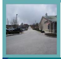
**Description:** Providing joint or cross access between adjacent properties allows circulation between the properties and reduces the number of driveways and conflict areas along a roadway. Joint and cross access can be used in combination with shared parking.
