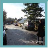
**Description:** A narrow roadway without pavement markings that is intended to support walking, biking, and driving in the low-speed travel way. These roads serve bi-directional traffic with no pavement markings, but their narrow design encourages lower speeds.
