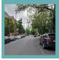
**Description:** Provision of on-street parking on one or both sides that reduces roadway width. Parked vehicles also provide a buffer between traffic and pedestrians on the sidewalk.
