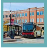
**Description:** Area adjacent and separate from the travel lanes on a roadway that provides space for buses to pick-up or drop-off passengers without impeding the flow of traffic. Bus bays are typically used on roadways with higher traffic volumes, higher speeds, or on congested corridors. They are also typically used for bus stops with higher ridership.
